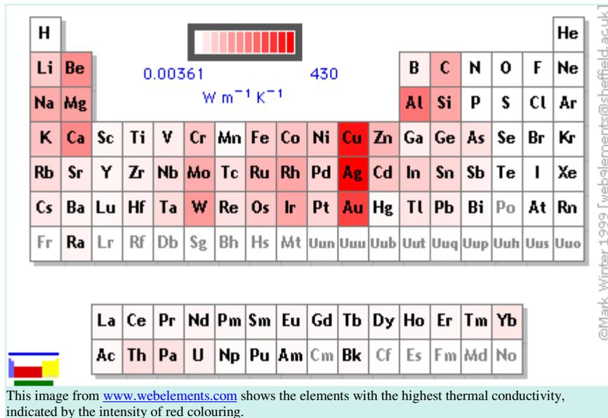
So what does all this mean? It means that heat energy from a processor die causes a variety of reactions on the atomic level within a heatsinks' material. Depending on what that heatsink is made of, it will have more or less resistance to moving that heat away to the surrounding air [mass](#). Understanding why metals are thermally conductive will hopefully explain a little bit about why copper is better than aluminum in this regard.
